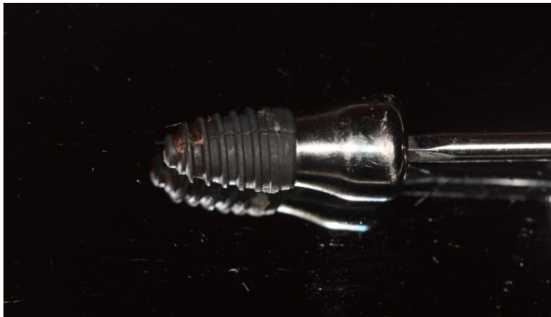
Figure 2. Vertical complete fracture of dental implant. Courtesy of Prof. Dr. Bruno Leitão de Almeida
