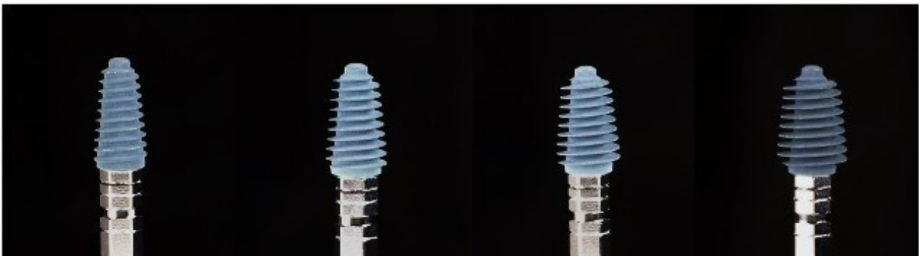
Fig 7. Example of implant samples used for our in vitro investigation. From left to right: implant 4mm (Group A), 4.5mm (Group B), 5mm (Group C), and 5.5mm (Group D) wide x 10 mm long.
