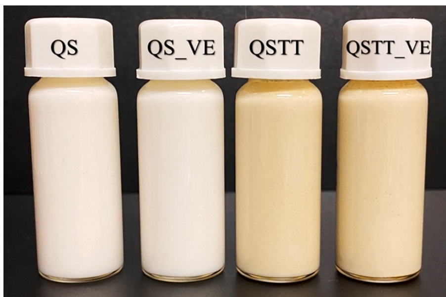
Fig. 1. Photo record of the produced nanoemulsions. The samples ‘QS’ and ‘QS_VE’ are the emulsions prepared using QS as the emulsifier, without and with VE, respectively. The samples ‘QSTT’ and ‘QSTT_VE’ are the emulsions prepared with the 50/50 QS/TT mixture as the emulsifier, without and with VE, respectively.
