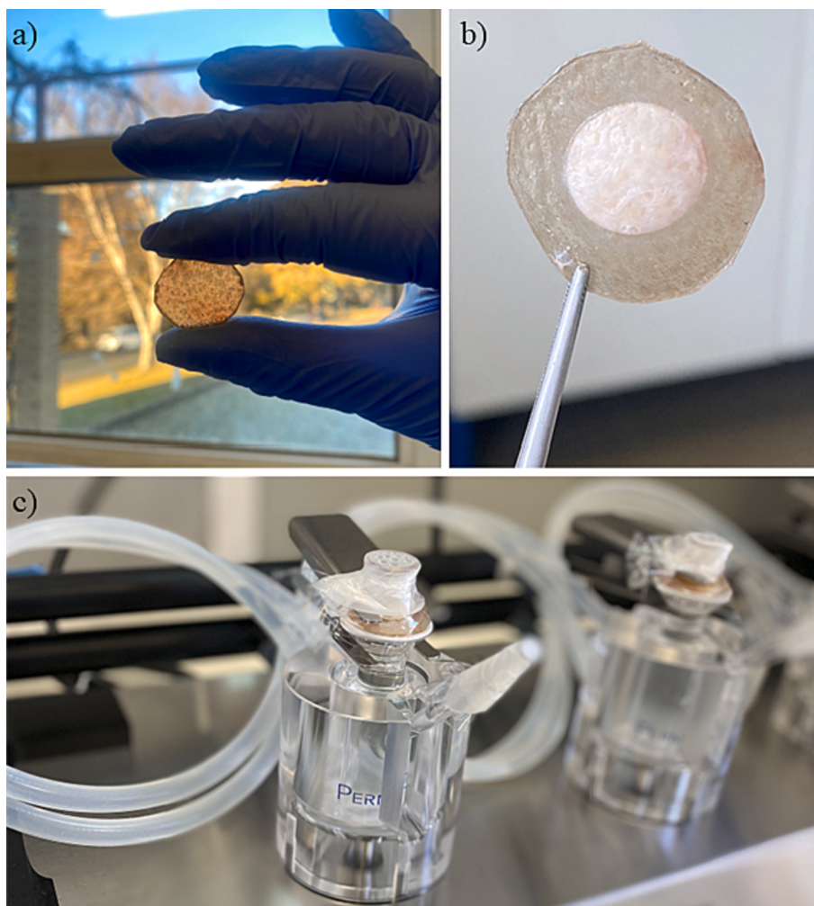
Fig. 6. Franz cell apparatus. a) Skin membrane before the experiment, b) Skin membrane after the experiment, c) Franz-cells during the experiment in occlusive conditions.
