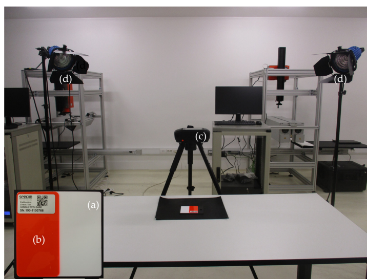
Figure 2. Experimental setup during the Specim IQ spectral range calibration check: (a) White reference and (b) calibration tile (SN: 190-110766), provided by the manufacturer (bottom left corner); (c) camera; (d) projectors with halogen lamps.
