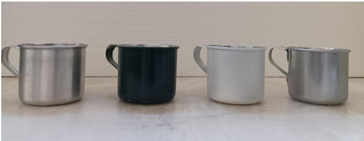
Figure 9. Aluminum cups used in cooling runs. From left to right: original and painted blackish green, white, and shiny silver.
