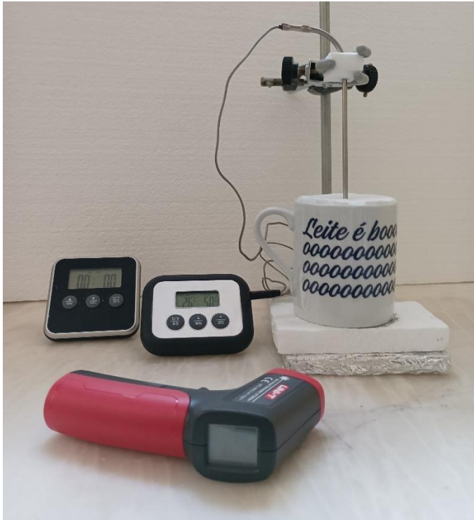
Figure 2. The set-up for carrying out the cooling experiments, showing the oven thermometer in place, the chronometer, and the IR thermometer used for reading the temperature of the outside surface temperature of the mug.
