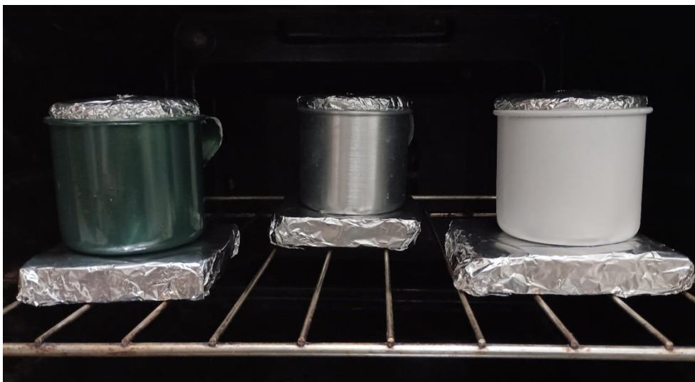
Figure 12. Aluminum cups filled with cold water and placed in a small conventional oven.
