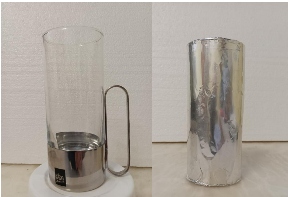
Figure 6. Glass mug with the removable hand and base on (left), and wrapped with aluminum foil (right), used in cooling experiments.
