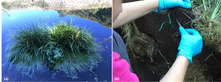
Figure 2. (a) Floating wetland island in a freshwater pond, (b) biofilm sampling for microbial communities analysis.
