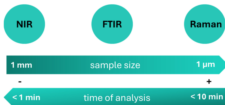
Figure 2. Time of analysis and sample size relations for the different vibrational spectroscopy techniques.
