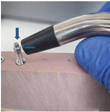
FIGURE 2 | Resonance frequency analysis (RFA) for stability. The secondary stability metric was measured using an Osstell device. A magnetic SmartPeg is attached to the implant, and the probe measures the implant stability quotient (ISQ) through noncontact resonance frequency analysis.
