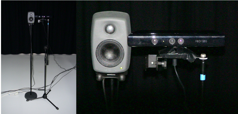
Figure 3.3: Left: a GENELEC 6010A loudspeaker (L2 in figure 3.2) with its main centre axis at the horizontal 0^\circ position and a Microsoft Xbox 360 Kinect depth camera. Right: a close-up of the same loudspeaker and the same camera with its infra-red projector (left), RGB camera (centre), and infra-red camera (right).
