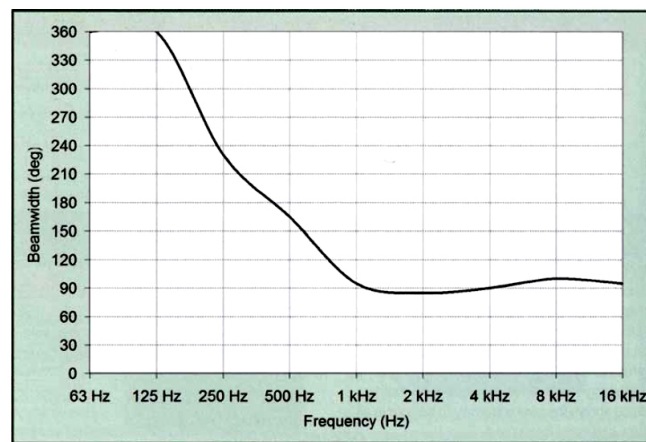
Figure 2.28: Beamwidth versus frequency of a loudspeaker with a nominal coverage angle of 90 degrees (McCarthy, 2007, p. 57).
