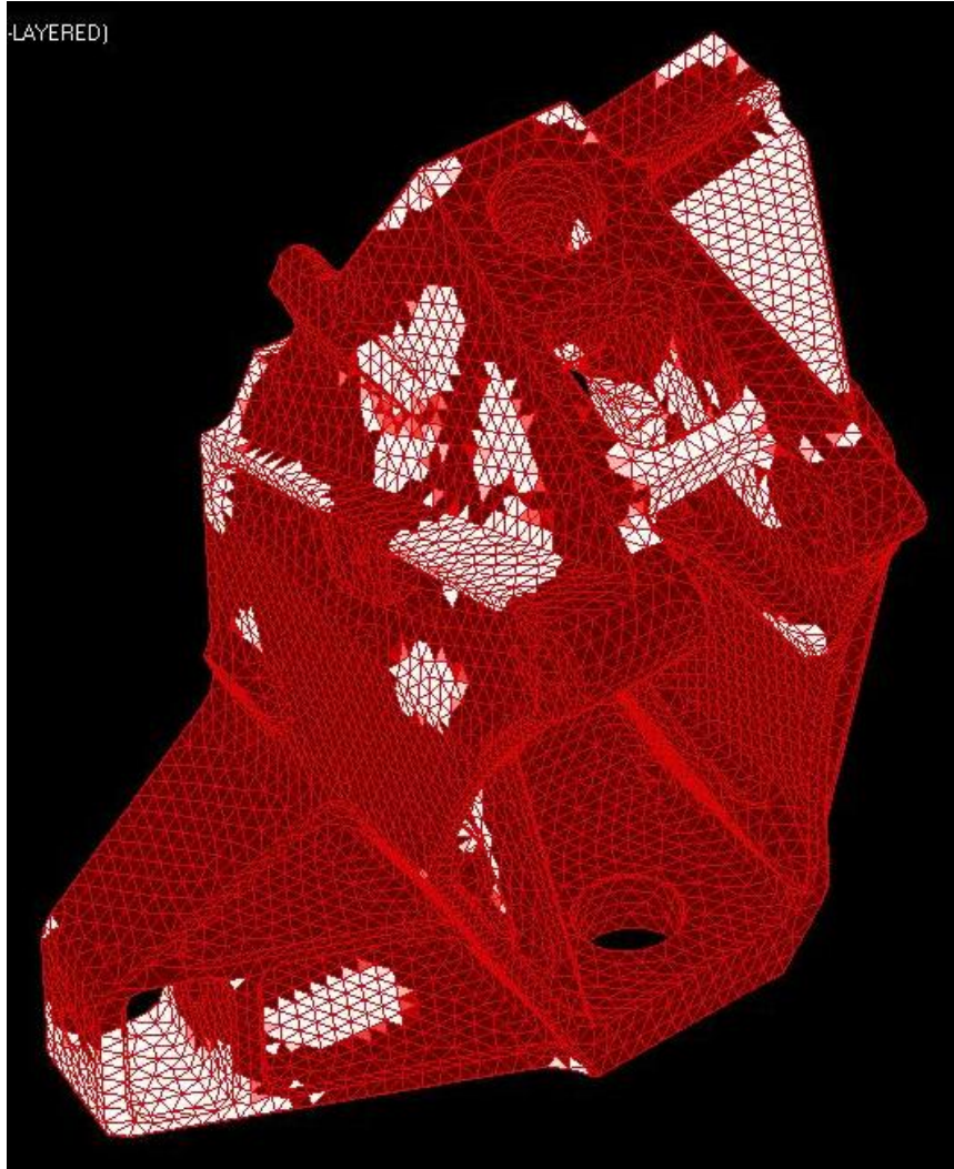
Figure 4-28 - Basic topology result for material reduction of 20% and threshold value of 0.0
