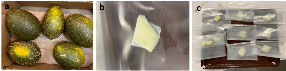
Figure 1 – Experimental procedure with melon samples: a) whole melon fruits purchased from a local Portuguese supermarket; b) melon slice (~3x3 cm) wrapped with the NC/ZnO film (5x5 cm); c) wrapped samples corresponding to one of the five experimental time points, stored in sterile bags for subsequent analysis.
