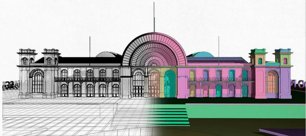
Fig. 16 - View of the original façade of the Crystal Palace modelled in the context of [Marca 3D] Project. The image shows a transition from a wireframe to a solid view to understanding the computer graphics process involved. © The authors
