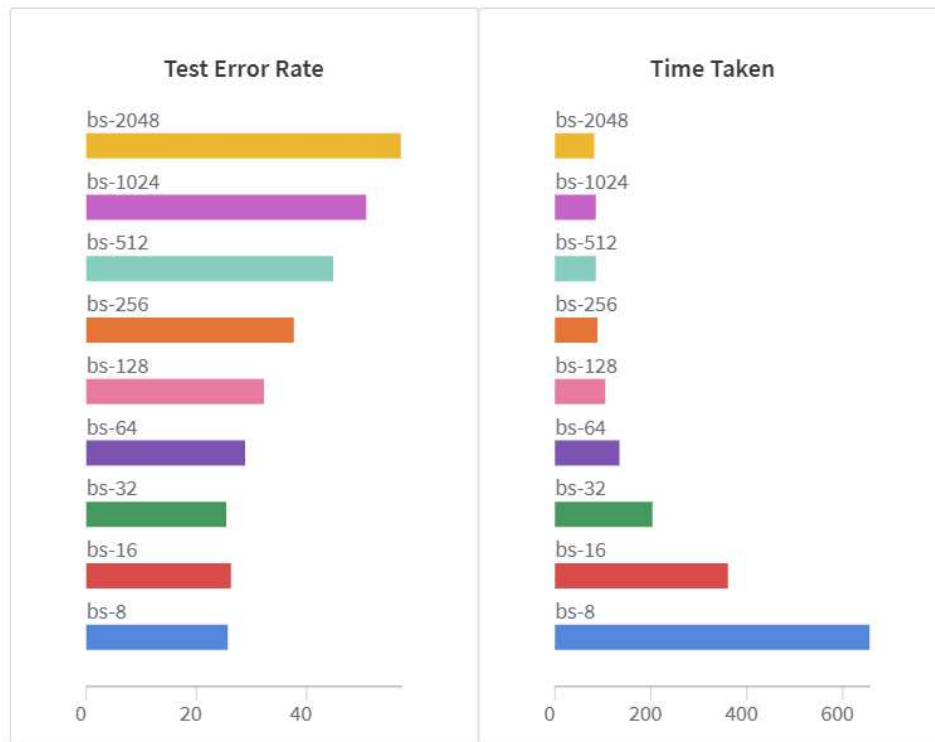
Figure 2.1 Test error rate and time taken for different batch sizes during neural network training. (Adapted from Ayush Thakur, 2025).
