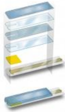
Figure 8 - Microfluidic test strip (Fontanazza, 2016).
