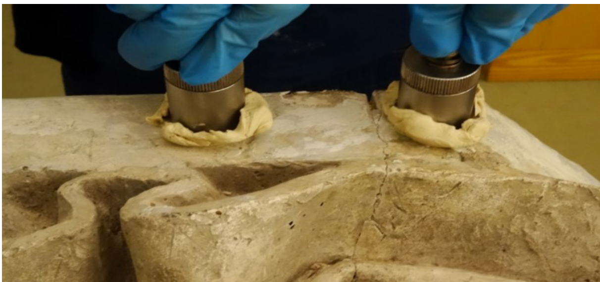
Figure 6 – A fracture at the base that has been repaired, but the signal is not transmitted through it. The white stain visible on the surface and inside the fracture is part of the repairing material.
