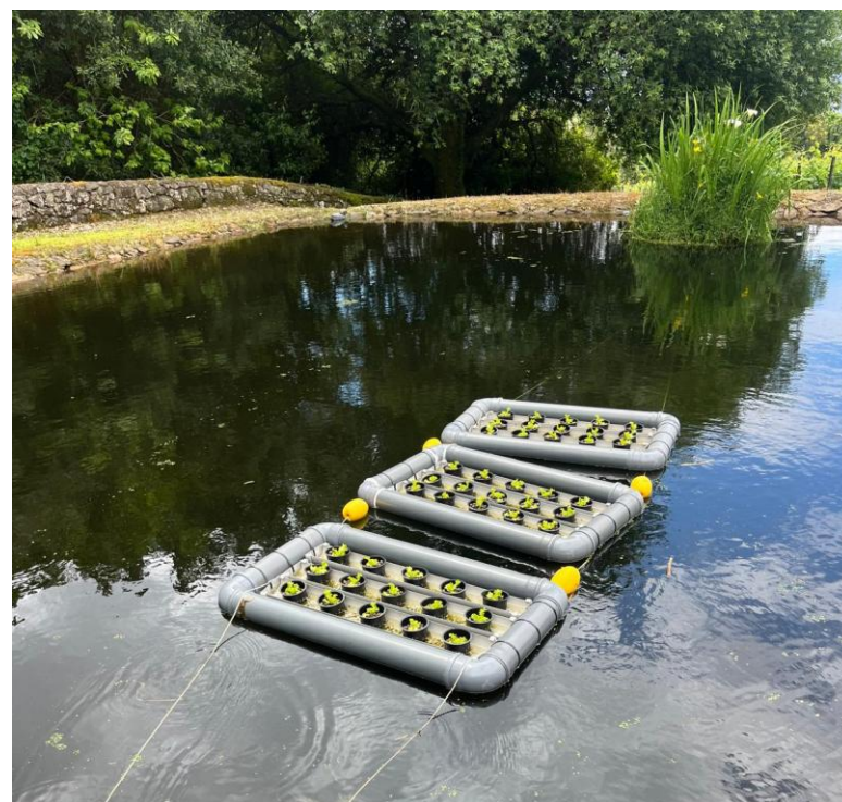
Figure 2. Experimental setup of the floating wetland islands at the study site.
