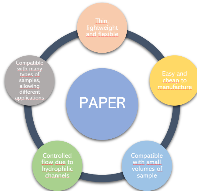
Figure 1.2 – Advantages of paper being used for fabricating \mu PAD, adapted from [33].
