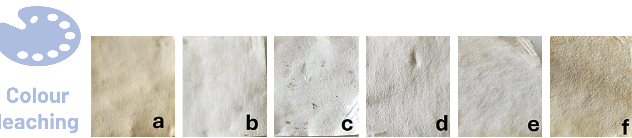
Figure 1. Photograph of white paper squares after 24 hours of incubation in contact with the different composites under a moistened cotton layer. a) control composite; b) composite containing elderberry bagasse; c) composite containing tomato marc; d) composite containing BSG; e) composite containing pear bagasse; f) composite containing apple bagasse.
