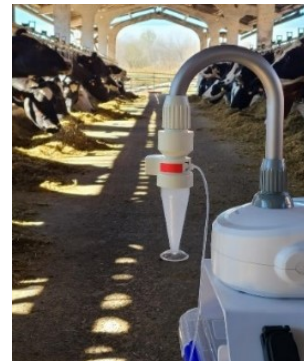
Figure 16 – Coriolis µ air-sampler (Bertin Technologies).
