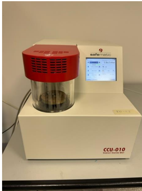
Figure 20 - Samples being sputter coated with gold.
