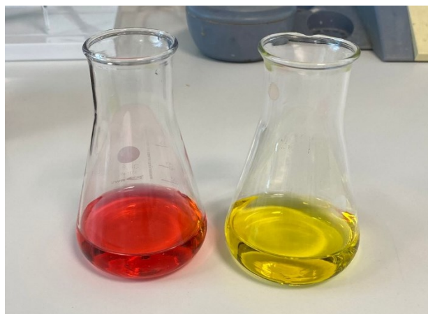
Figure 11- H 2 SO 4 titration with NaOH, changing the red from methyl red to yellowish colour.
