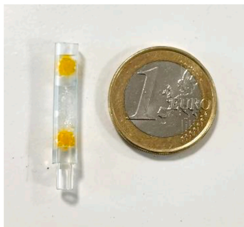
Fig. 1. Photograph of the Chelex 100 packed column alongside a one-euro coin for scale.
