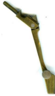
Figura 73- Ponta de lápis para compasso. National Museum of American History. (Fonte: https://americanhistory.si.edu/collections/search/object/nmah_904352 )
