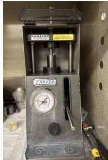
Figure 2. Carver Press Machine for Zirconia Green body Preparation. The image shows the machine with a zirconia powder in the mold, where it is subjected to a pressing force of 1 ton for 5 min.
