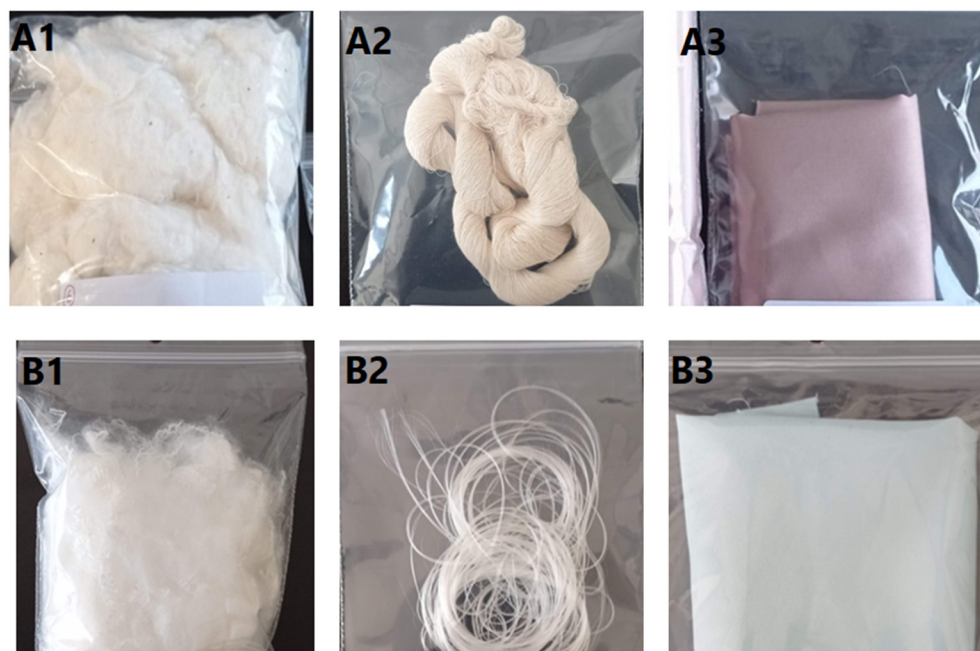
Figure 5. Pictures of 100% cotton (A1—raw; A2—yarn; A3—fabric) and 100% polyester (B1—raw; B2—yarn; B3—fabric) samples.
