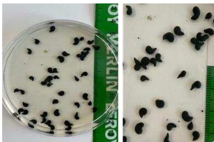
Figure 11 - Multi-immobilized bacteria granules produced through the co-immobilization of strains Labrys portucalensis F11, Rhodococcus sp. S2, and Rhodococcus sp. ED55 in an EPS matrix.
