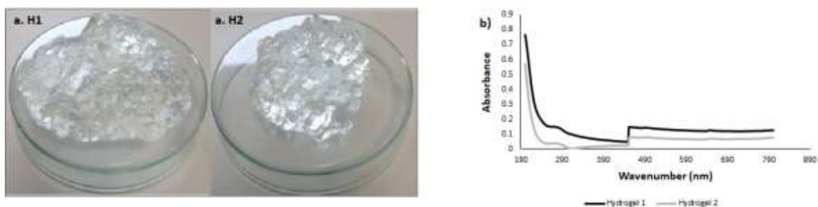
Figure 1. Images of aH1) cellulose-based hydrogel synthesized using natural cellulose fibers extracted from sugarcane bagasse (H1) and of aH2) cellulose-based hydrogel synthesized using commercial cellulose from Sigma-Aldrich (H2). b) Absorbance profile of Hydrogels H1 and H2.
