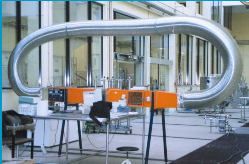
Pilot plant tray drier (Armfield UOP8).
