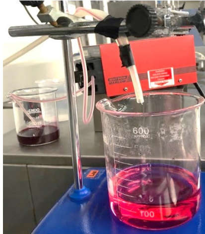
Figure 4.2- Assembled system for the formation of alginate capsules with dye using compressed air. The alginate aqueous solution is being fed to the peristaltic pump, which is connected to a syringe attached to the compressed air hose. Smaller capsules are then formed when the droplets come into contact with the calcium chloride solution from the beaker below it.
