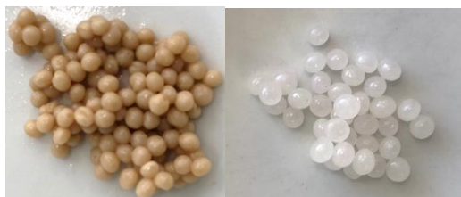
Figure 5.6- Shellac-alginate (on the left) and alginate (on the right) capsules with sunflower oil, made by ionic gelation, using the syringe method.
