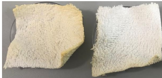
Figure 5.24- Impregnation of the alginate capsules with Aloe vera extract, corresponding to sample 21 (on the right), and of the alginate capsules made with the same method, representing sample 22 (on the left). Both impregnation solutions containing Tubicoat HEC at the concentration of 2.5% w/v and 1.25%w/v, for sample 21 and 22 respectively.
