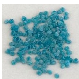
Figure 5.1- Alginate capsules with food colouring made by ionic gelation, after the drying process.
