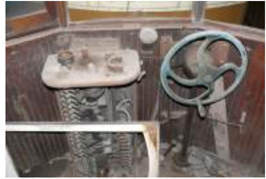
Fig. 4 - Detail of one controller.
