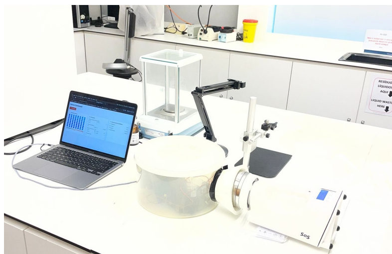
Figure 4. Experimental validation setup. The acrylic chamber isolates the sensor array and the biological culture. The integrated fan system creates a turbulent flow, forcing the aerosolization of spores.
