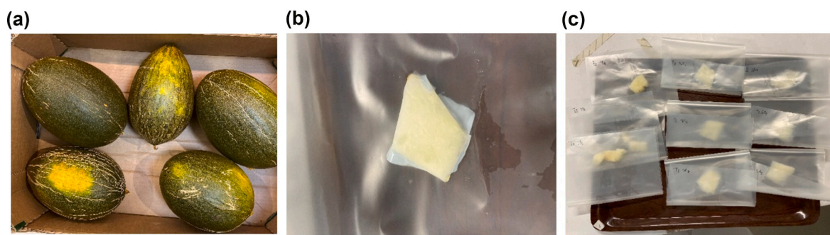
Fig. 1. – Experimental procedure with melon samples: a) whole melon fruits purchased from a local Portuguese supermarket; b) melon slice ( \sim 3 \times 3 cm) wrapped with the NC/ZnO film ( 5 \times 5 cm); c) wrapped samples corresponding to one of the five experimental time points, stored in sterile bags for subsequent analysis.
