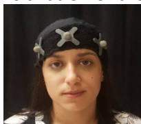
Figure 11: Fabric helmet with sensors for data collection
