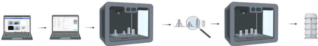
Figure 20 - 3D printing process of the Tunnel Filler
