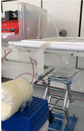
Figure 11 - Engineered mechanism to produce Pcl electrospun fibers with the best dispersion possible
