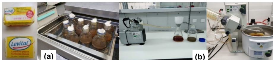
Fig. 3. (a) Applied yeast and fermentation in a thermostatic bath with slow shaking; (b) Vacuum filtration and ethanol recovery using a rotary evaporator.
