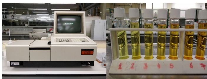
Fig. 4. UV-Vis spectrophotometer (left) and the standards used to prepare the calibration curve (right).
