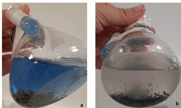
Figure 5.8 – Batch liquid cultures containing heat-inactivated aerobic granules in SBR medium with Navy Everzol ED dye ([NE] = 7.5 mg/L). a) shows the beginning of the experiment with blue colored flask; b) experiment after 24/48 hours with colorless flask and colored granules.
