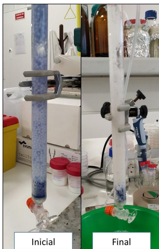
Figure 4.6 - Decolorization of simulated effluent of Navy Everzol ED (6x diluted) in a preparative column using yeast Y. lipolytica (HOMOGST27A) capsules.
