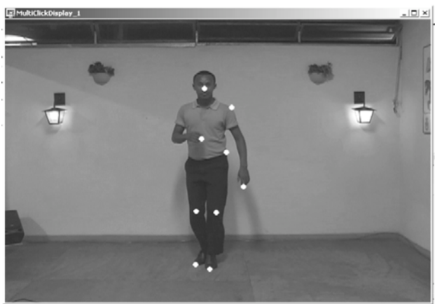
Fig. 5. Frame-by-frame manual tracking. Each white dot represents one position marked with the mouse using visual identification (the size of the points shown here is bigger than the original to facilitate visualization). The original patch offers a visually recognizable mark definition of 1x1 pixel along a spatial definition of DV format (720x480 pixels).
