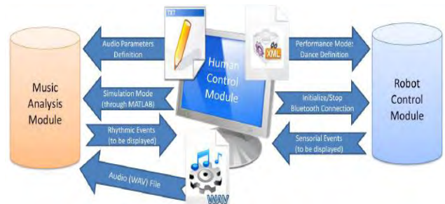
Fig. 6 Human Control Module (GUI) bi-directional interaction with the Music Analysis Module and the Robot Control Module.
