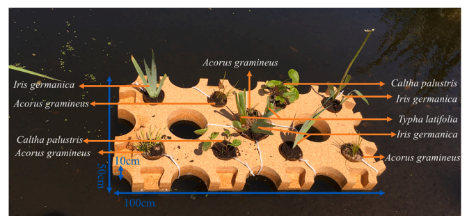
Fig. 1. Floating treatment wetland configuration setup with platform dimensions (100 × 50 × 10 cm) and plant species: Iris germanica (4 plants), Caltha palustris (2 plants), Acorus gramineus (4 plants), and Typha latifolia (2 plants).
