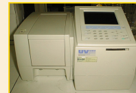
Determination of optical density at 560nm (O.D. 560 ) every hour for the first 8h, and by 24h (Taranto et al. , 1996)
