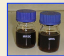
Inoculation into MRS broth and MRSO broth (containing 0.3% Oxgall), and incubation at 37°C / 24 h
